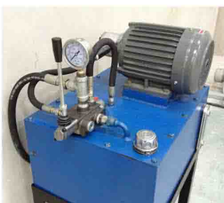
Hydraulics assembly with nonflammable hydraulic fluid
